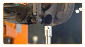
Unscrew the lower fastener of the shock absorber. Use a drive socket #14.
