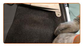
Install the clips of the boot side lining.
