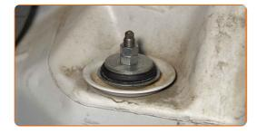
Unscrew the upper fastener of the shock absorber. Use a combination spanner #14 (2 pieces). Use a shock absorber socket DD#6.
