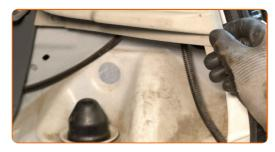
Remove the mount cap from the shock absorber upper fastener.
