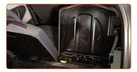
Remove the clips of the boot side lining. Use a clip removal tool.
