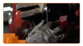
10 Remove the brake caliper.
