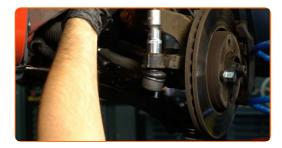
Screw on the tie rod end jam nut. Use a combination spanner #17. Use a combination spanner #19.
