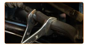
Tighten the tie rod end locknut. Use a combination spanner #17. Use a combination spanner #19. Use a torque wrench. Tighten it to 47 nm torque.
