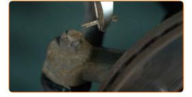
Clean the fastener connecting the tie rod end to the steering knuckle. Use a wire brush. Use WD-40 spray.
