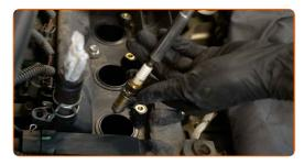
Apply a thin layer of a special high temperature anti-seize lubricant to the threads of the new spark plugs. Use a flat screwdriver.
