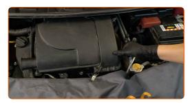
Install the fastening clamps of the air filter breather pipe and the air filter inlet pipe. Use clic-R collar pliers.
