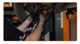
13 Remove the fastening bolt.
