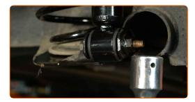
Tighten the lower fastener of the shock absorber. Use a drive socket #14. Use a torque wrench. Tighten it to 48 Nm torque.
