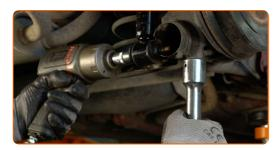
Screw the upper fastener of the shock absorber.
