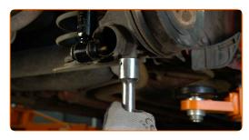
Screw in the lower fastener of the shock absorber. Use a drive socket #14.
