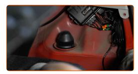
Unscrew the upper fastener of the shock absorber. Use a combination spanner #14 (2 pieces).
