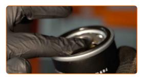
Screw the new filter into its place. Use the 67-14F socket. Use a torque wrench. Tighten it to 23 Nm torque.
