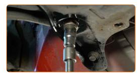
17 Remove the rear fastener of the control arm. Use a drive socket #17.
