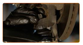
Tighten the rear fastener of the control arm. Use a drive socket #17. Use a torque wrench. Tighten it to 100 Nm torque.
