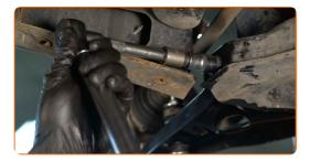
Tighten the ball joint fastener. Use a combination spanner #19. Use a torque wrench. Tighten it to 98 nm torque.
