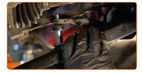
Screw in the fastener connecting the stabilizer bar to the control arm. Use a combination spanner #10. Use a drive socket #12. Use a ratchet wrench.
