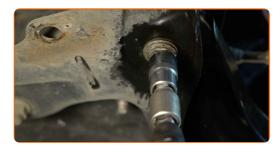
Tighten the front fastener connecting the control arm to the subframe. Use a drive socket #17. Use a torque wrench. Tighten it to 116 Nm torque.
