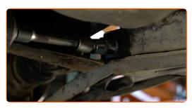
Remove the front fastener of the control arm. Use a drive socket #17.
