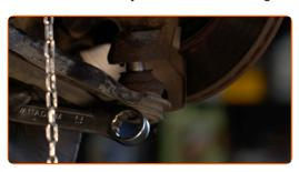
Disconnect the lower arm from the steering knuckle.
