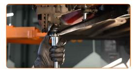
Tighten the ball joint fastener. Use a combination spanner #19. Use a torque wrench. Tighten it to 98 nm torque.
