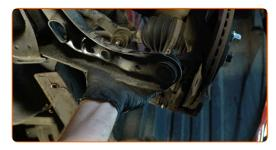
Unscrew the fastener connecting the stabilizer link to the stabilizer bar. Use a combination spanner #10. Use a drive socket #12. Use a ratchet wrench.
