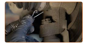
Clean the fastener connecting the ball joint to the steering knuckle. Use a wire brush. Use WD-40 spray.
