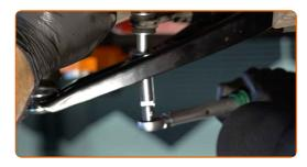
Remove the support from under the arm.
