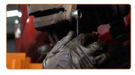
10 Remove the brake caliper.
