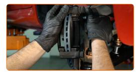
Tighten the brake caliper bracket. Use a drive socket #17. Use a torque wrench. Tighten it to 89 Nm torque.
