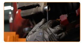
10 Remove the brake caliper.
