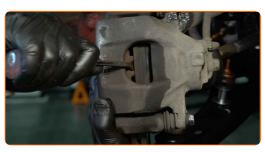
Unscrew the brake caliper fastening. Use a drive socket #13. Use a ratchet wrench.
