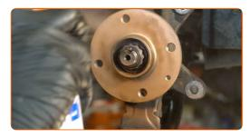
19 Install the brake disc.
