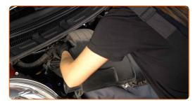
6 Cover the throttle body with a microfibre towel to prevent dust and dirt from getting into the system.
