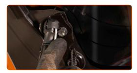
Unscrew the fastener of the boot side lining. Use a Phillips screwdriver.
