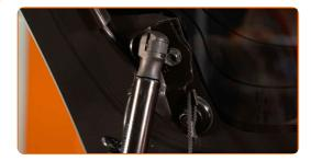
Screw in the fastener of the boot side lining. Use a Phillips screwdriver.
