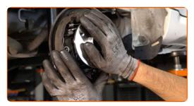
Tighten the fastener of the wheel hub bearing. Use a drive socket #12. Use a torque wrench. Tighten it to 60 nm torque.
