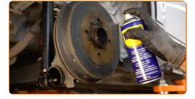
Unscrew the brake drum fastening. Use Torx T30. Use an impact screwdriver.
