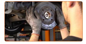
Tighten the brake drum fastener. Use Torx T30. Use a torque wrench. Tighten it to 5 Nm torque.
