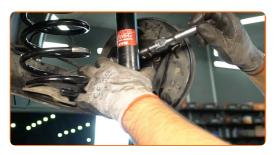
Replacement: wheel bearing – PEUGEOT 107 Hatchback (PM, PN).
