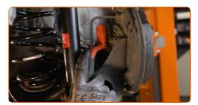
Unscrew the ABS sensor fastener. Use Torx T30. Use a ratchet wrench.
