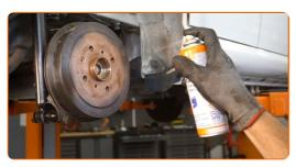
Treat the fasteners of the wheel hub bearing. Use copper grease.
