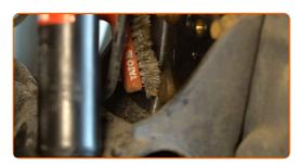
Unscrew the hub bearing mounting. Use a drive socket #12. Use a ratchet wrench. Use a tap wrench.
