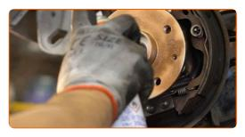
Install the brake drum and fasten it.
