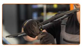
Remove the blade from the wiper arm.
