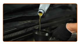
Replacement: engine oil and filter – PEUGEOT 106 II Hatchback (1A, 1C). Tip from AUTODOC experts:
