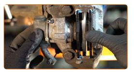
Replacement: brake pads – PEUGEOT 106 II Hatchback (1A, 1C). Tip:
