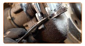
Remove the brake pads. Use a crowbar.
