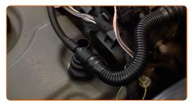
Remove the crankcase ventilation hoses.
