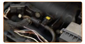
Connect the crankcase ventilation hose to the intake manifold.
