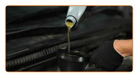
Replacement: engine oil and filter – PEUGEOT 106 I Hatchback. Tip from AUTODOC experts:
