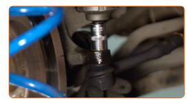
Screw on the tie rod end jam nut. Use a combination spanner #22 (2 pieces).
