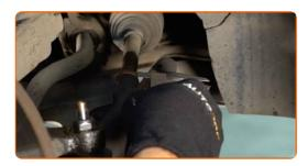
Tighten the tie rod end locknut. Use a combination spanner #22 (2 pieces). Use a torque wrench. Tighten it to 50 nm torque.
