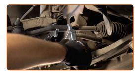
Tighten the fastening nut connecting the tie rod end to the steering knuckle. Use a drive socket #17. Use a torque wrench. Tighten it to 38 nm torque.
