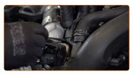
3.2 Squeeze the clamp with combination pliers and disconnect the vacuum valve hose.
