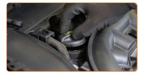
Pour oil into the engine through the filler. Required amount of oil: 4.25 l.
