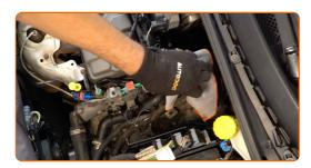
Reinstall the air filter housing.
