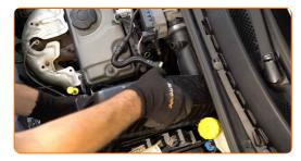
Screw the filter housing fastening bolts. Use a drive socket #10. Use a ratchet wrench.
