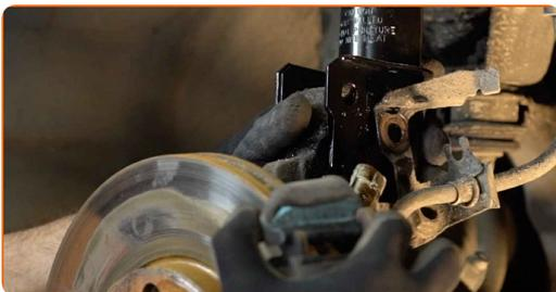
**32** Install the new steering knuckle bolts.
