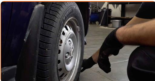
45 Remove the fender protection cover.
