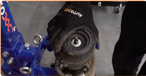
24 Install the new mount, boot, and bump stop on the shock absorber.
