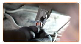
Clean the oxygen sensor fastener. Use a wire brush. Use WD-40 spray.
