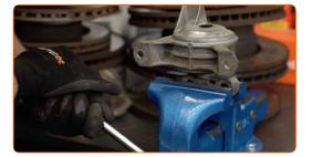
Unscrew the engine mount from the bracket. Use Torx T55. Use a ratchet wrench.
