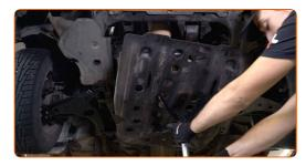
Support the engine skid plate. Use a hydraulic transmission jack.
