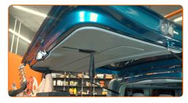
Unscrew the fastener of the third brake light. Use an 8 mm socket. Use a ratchet wrench.
