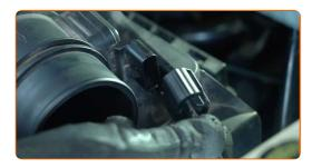
Unscrew the air filter cover fasteners. Use a T25 Torx screwdriver.
