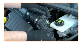
Tighten the clamp of the air intake hose. Use a 7 mm socket. Use a ratchet wrench.
