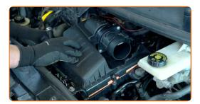
Tighten the air filter cover fasteners. Use a T25 Torx screwdriver.
