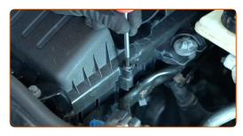
Treat the connector of the MAF sensor. Use an electronic spray.
