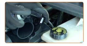
Reattach the connector to the MAF sensor.
