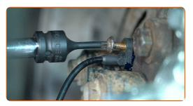
Tighten the ABS sensor fastener. Use a T30 Torx bit. Use a torque wrench. Tightening torque: 8 N·m.
