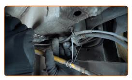
Clean the ABS sensor mounting seat. Use a wire brush. Use an all-purpose cleaning spray. Use a wire bore brush drill attachment.
