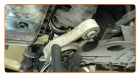
Replacement: engine mounts – OPEL Vivaro A Platform / Chassis (X83).
