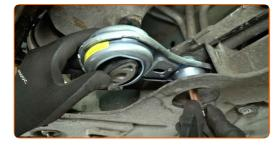
Tighten the fastener that connects the engine mount to the engine mount bracket. Use a 24 mm socket. Use a torque wrench. Tightening torque: 100 N·m.
