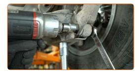
Unscrew the upper fastener of the shock absorber. Use a 21 mm combination spanner. Use a 21 mm socket. Use a ratchet wrench.
