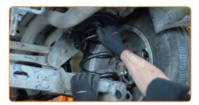
Jack up the rear axle beam. Use a transmission jack or one more vehicle jack.
