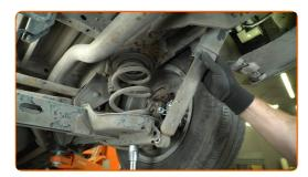
Carefully lower the transmission or vehicle jack to release tension from the spring.
