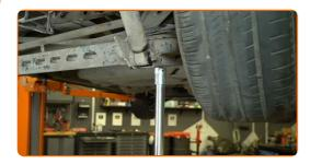
Unscrew the lower fastener of the shock absorber and remove the stop plate. Use a 21 mm combination spanner. Use a 21 mm socket. Use a ratchet wrench.
