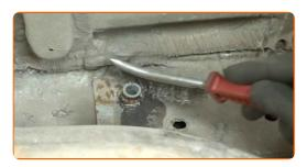
Clean the spring mounting seats. Use a wire brush. Use an all-purpose cleaning spray.
