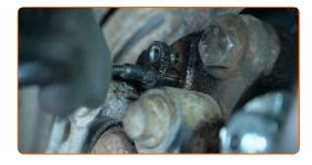
6.1 Detach the ABS sensor wiring.
