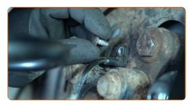
Remove the ABS sensor. Use a mounting lever.
