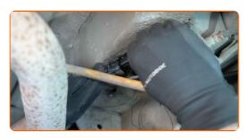
11 Secure the ABS sensor wiring.
