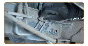
6.2 Detach the vehicle connector from the ABS sensor connector.
