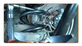
Remove the fastening bolt.
