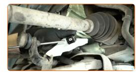
Secure the ABS sensor connector in its mounting seat on the vehicle.
