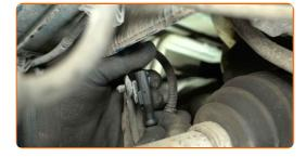
Attach the vehicle connector to the ABS sensor connector.
