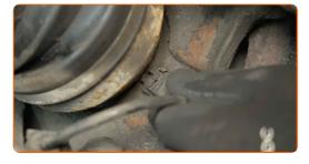
Detach the ABS sensor wiring.
