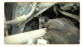
Treat the vehicle connector of the ABS sensor. Use an electronic spray.
