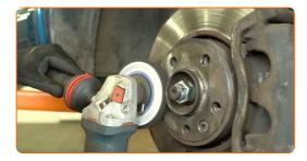
Treat the brake disc surface that contacts the wheel rim. Use ceramic grease.
