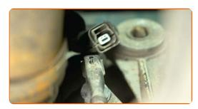
Remove the ABS sensor connector from its mounting seat on the vehicle. Use a slotted screwdriver.
