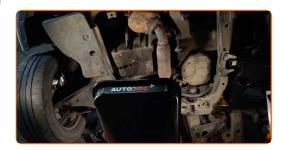
Clean the area of the oil pan drainage hole. Use a wire brush. Use all-purpose cleaning spray.
