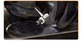
Install the retainers of the fasteners of the fuel filter tubes.
