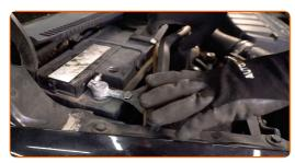
Screw in the fastener of the wiper cowl grille located on the left side. Use Torx T25.
