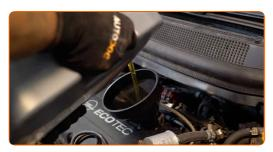
Replacement: engine oil and filter – OPEL Vectra C CC (Z02). AUTODOC recommends:
