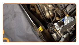
Remove the oil filler cap. Insert the funnel.
