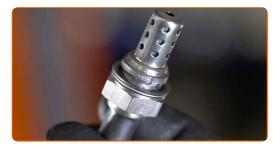
10 Install the new oxygen sensor.
