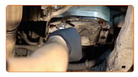
10 Remove the transmission fluid pan.
