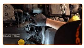
Return the coolant pipe to its initial position and fasten it.
