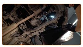
Unscrew the fasteners of the transmission fluid pan. Use a drive socket #11. Use a ratchet wrench.
