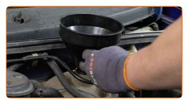
Pour coolant in the coolant reservoir.
