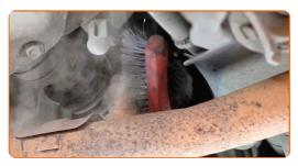
Detach the oxygen sensor connector.
