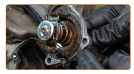
Cover the mounting seat of the thermostat housing with a microfibre cloth to prevent dirt and foreign objects from entering the system.
