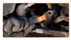
Install a new rod, tighten the fasteners.
