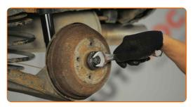
9 Remove the brake drum.
