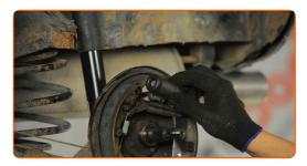
Tighten the wheel cylinder fastener. Use a drive socket #10. Use a torque wrench. Tighten it to 10 nm torque.
