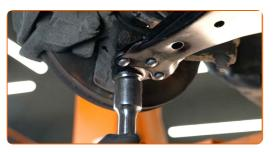
Screw the fasteners of the ball joint. Use a combination spanner #18. Use a drive socket #18. Use a ratchet wrench.
