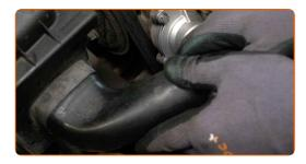
Attach the clip on the air filter intake hose.
