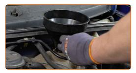
Pour coolant in the coolant reservoir.
