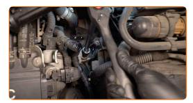
Insert the funnel. Pour new transmission fluid in the gearbox through the breather hole. Required amount of oil: 1.6 L.
