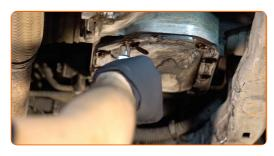
10 Remove the transmission fluid pan.
