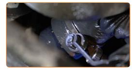
Secure the coolant hose clamp. Use clic-R collar pliers.
