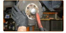
Unscrew the brake drum fastening Use Torx T30. Use a ratchet wrench.
