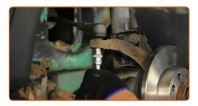
Tighten the tie rod end locknut. Use a combination spanner #19. Use a torque wrench. Tighten it to 50 nm torque.
